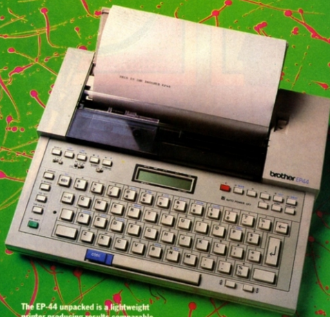
The EP-44 unpacked is a lightweight printer producing results comparable to daisywheel printers.
